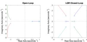
Here the open-loop system features both a non-minimum phase zero and an unstable pole. When looking at the left half of the symmetric root locus, the mirrored NMP zero and mirrored unstable pole stabilize the system such that for any  $\rho$  the closed loop poles will stay on the LHP.
