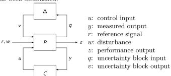
The objective is to stabilize the system in presence of  $\Delta$  and minimize the performance outputs z, given the exogenous reference and disturbances.
