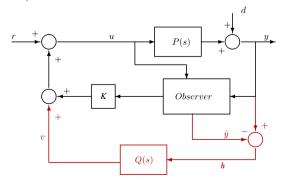
Assuming a controllable and observable plant, the closed-loop
