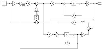
Like with the LQR compensator an integrator can be added
