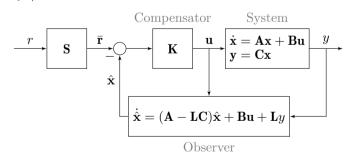
The closed-loop system is given by
